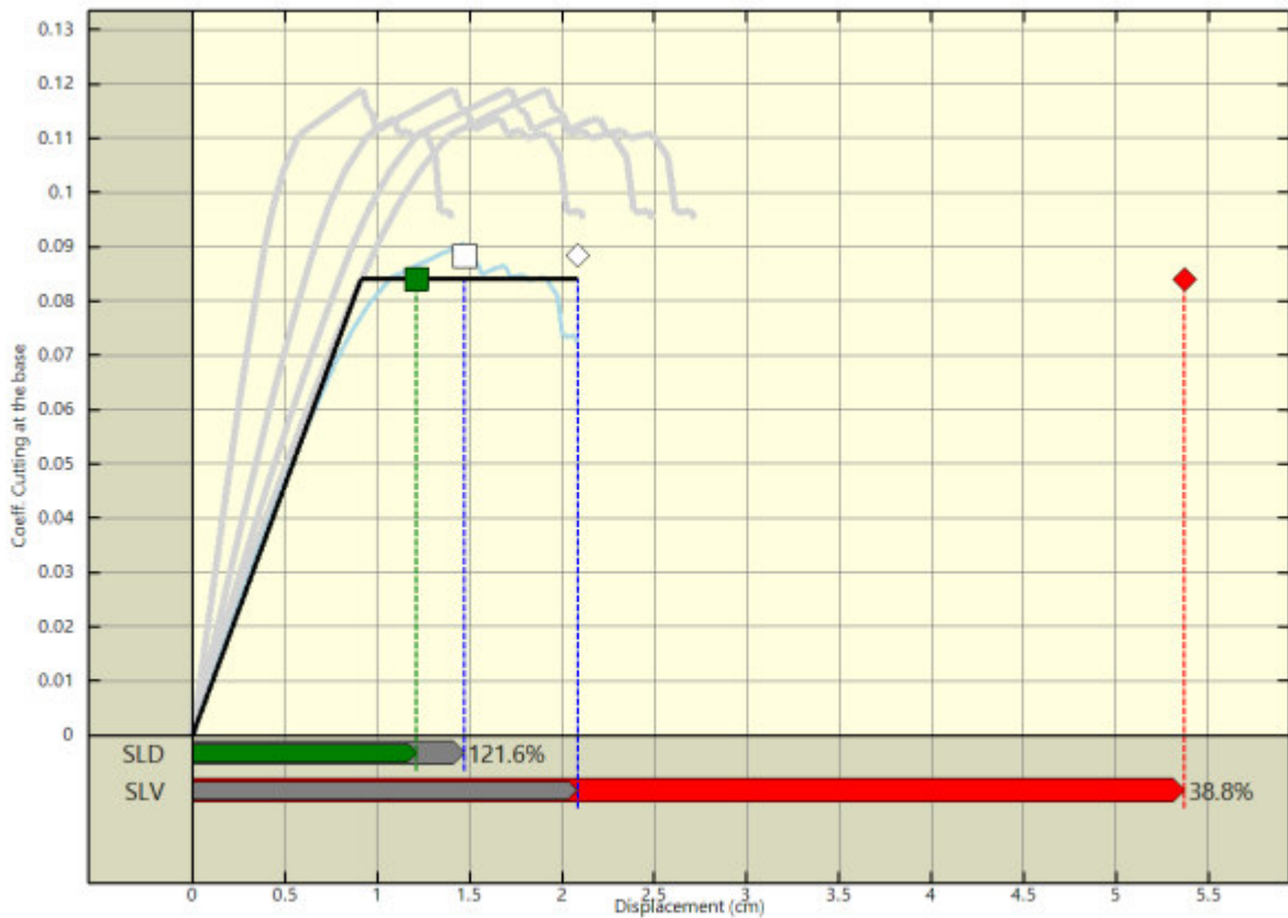
Pushover analysis "Pushover -X Massa + e" : seismic vulnerability assessment.
